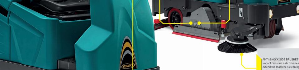
Impact resistant side brushes extend the machine's cleaning path, reaching hard to access spots and under low profile objects.
