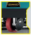
DRIVE MOTOR PROTECTED AGAINST IMPACT AND WATER The motor drives the front wheel via a lubricated gearbox. Installed vertically inside the nose of the machine this position delivers maximum protection
