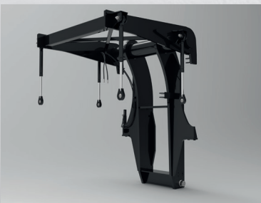
Gantry carriage 750 for top pick 20'-40' telescopic spreader 818 with Mechanical Pile Slope.
