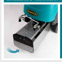
Close cleaning right up until the escalators balustrade, independent of the width of the steps.
