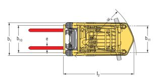
$$\label{eq:asymptotic_state} \begin{split} & \text{Ast=W}_{\text{a}} + \text{SQRT} \; \{ (\text{I}_{\text{6}} + \text{x})2 \; + \; (\text{b}_{\text{12}} / 2 \cdot \text{b}_{\text{13}} )2 \} + \text{a} \\ & \text{a} = \text{minimum operating clearance} \\ & \text{(VDI standard} = 200 \; \text{BITA recommendation} = 300 \text{mm)} \\ & \text{I}_{\text{6}} = \text{Load length} \end{split}$$
