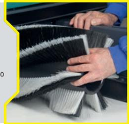
The retractable, anti-shock side brushes (AMSD system - a Eureka patent) enable the Rider 1201 to sweep in confined areas and under low profile objects.
