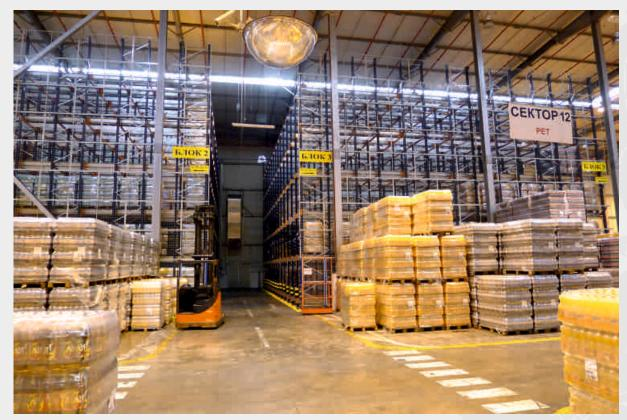
**COCA COLA** company, Bulgaria Stage 3, total of 2 520 p.p. 14 lanes, 6 levels, 30 pallets in depth 4 shuttle cars LIFO
